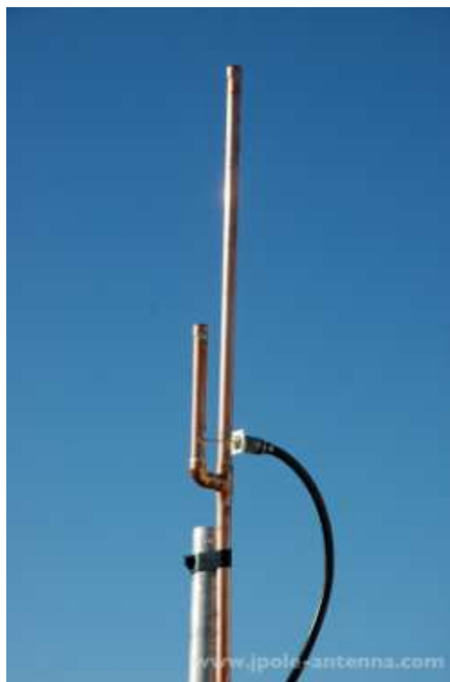
Copper pipe J-Pole Antenna
