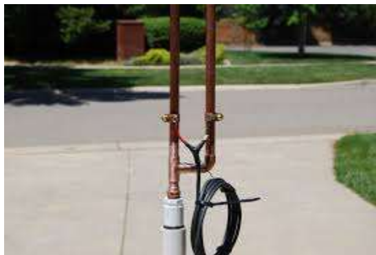
Direct feed with coax choke balun.
