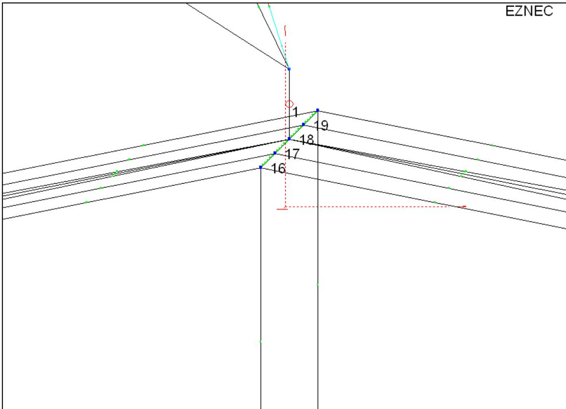
The graphic above shows how the feed point is modeled. I defined a single one foot long vertical wire with its bottom end connected to the center of the roof. I then instructed EZNEC to install an RF source in the middle of that short wire. The three quarter wave wires then connect to the top end of this wire. This is a common way of modeling multiple wires fed from a single source.
