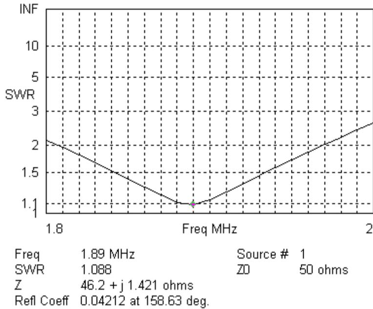
The SWR plot above shows more detail for the 160-meter band. It was a surprise how low the SWR is at resonance and how broad the SWR curve is. My guess is that this is a result of ground losses. My biggest surprise was that a plot made with my SWR bridge exactly matches the EZNEC plot.
