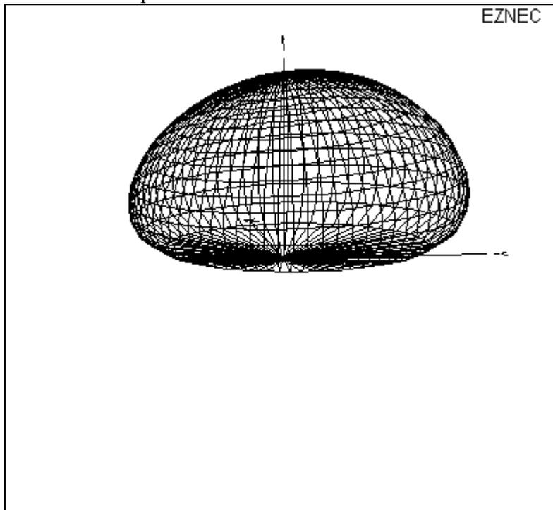
The graphic above is what EZNEC thinks the radiation pattern should be on 160 meters. Notice that because of the slope of the wire, there is no overhead null as would be found on a pure vertical antenna. EZNEC shows the gain of this antenna as  $-2.94$  dBi.
