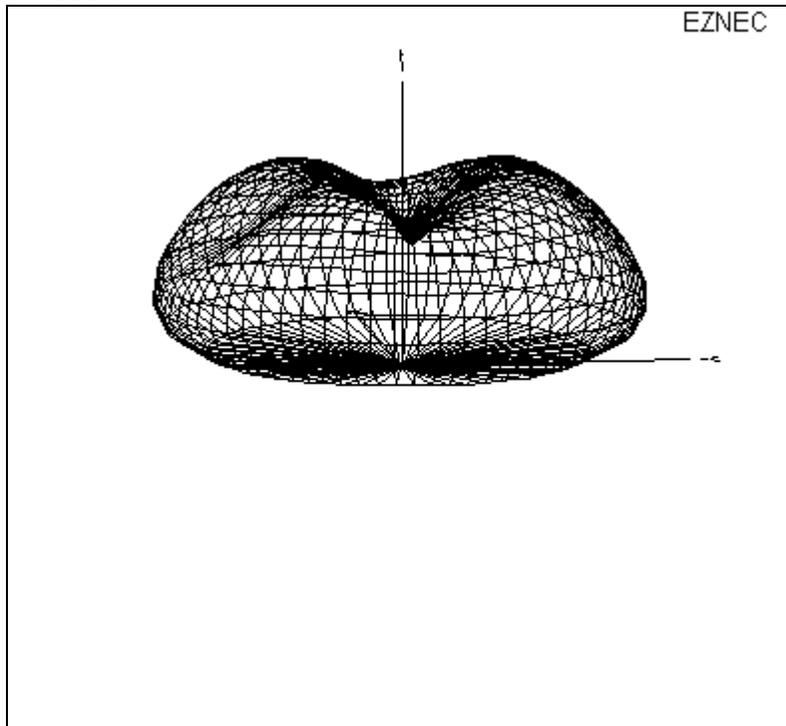
The graphic above is of the 40-meter radiation pattern. EZNEC indicates the gain at this frequency is 0.12 dBi. Some interaction with the 160-meter and/or the 75-meter wire is
