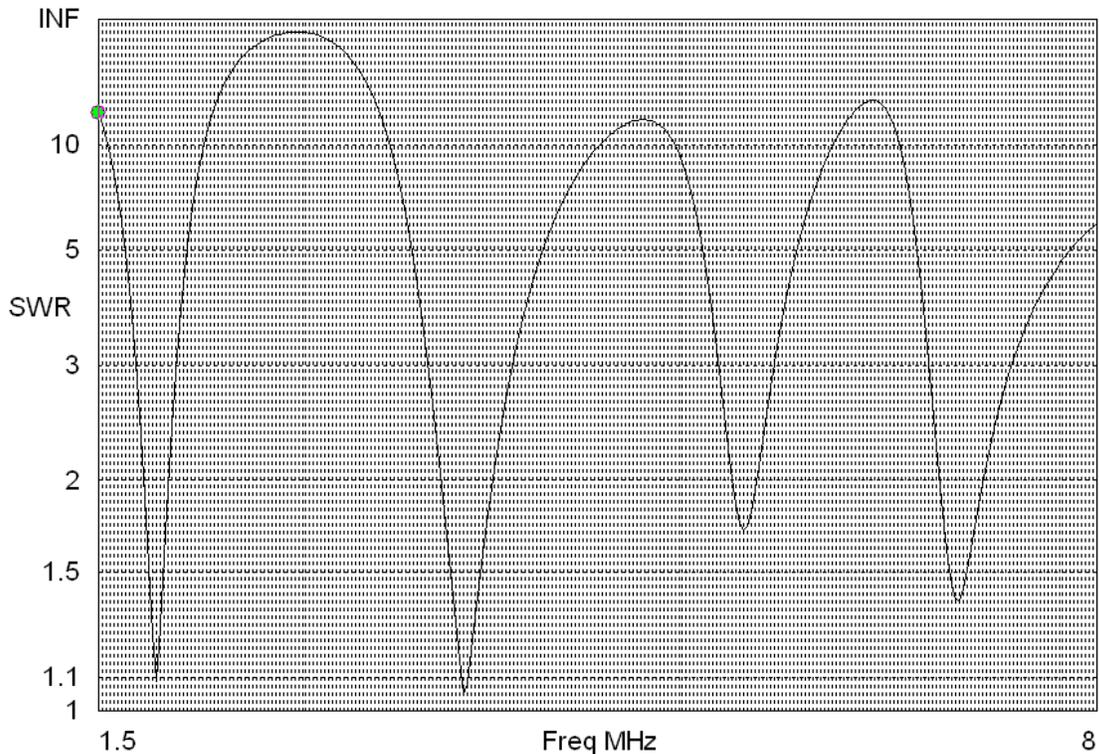
The SWR plot above is EZNEC's estimation for the entire range of 1.5 MHz through 8 MHz. The SWR dips occur at 1.9 MHz, 3.8 MHz, 5.6 MHz and 7.2 MHz. The SWR dips in 160 meters, 75 meters, and 40 meters are from the three wires attached to the common feed point. The 5.6 MHz dip is the third harmonic of the 1.9 MHz wire.
