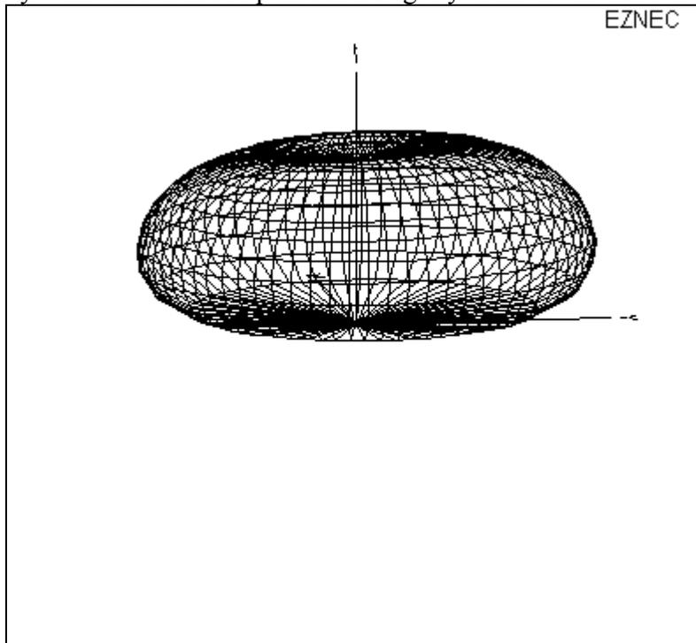
The 3 dimensional radiation plot above for 75 meters shows a typical Inverted-L pattern. There is a little bit of a null overhead. The slope of the vertical wire and the horizontal tail fill in so a perfect null is not produced. EZNEC shows the gain as 0.57 dBi.
