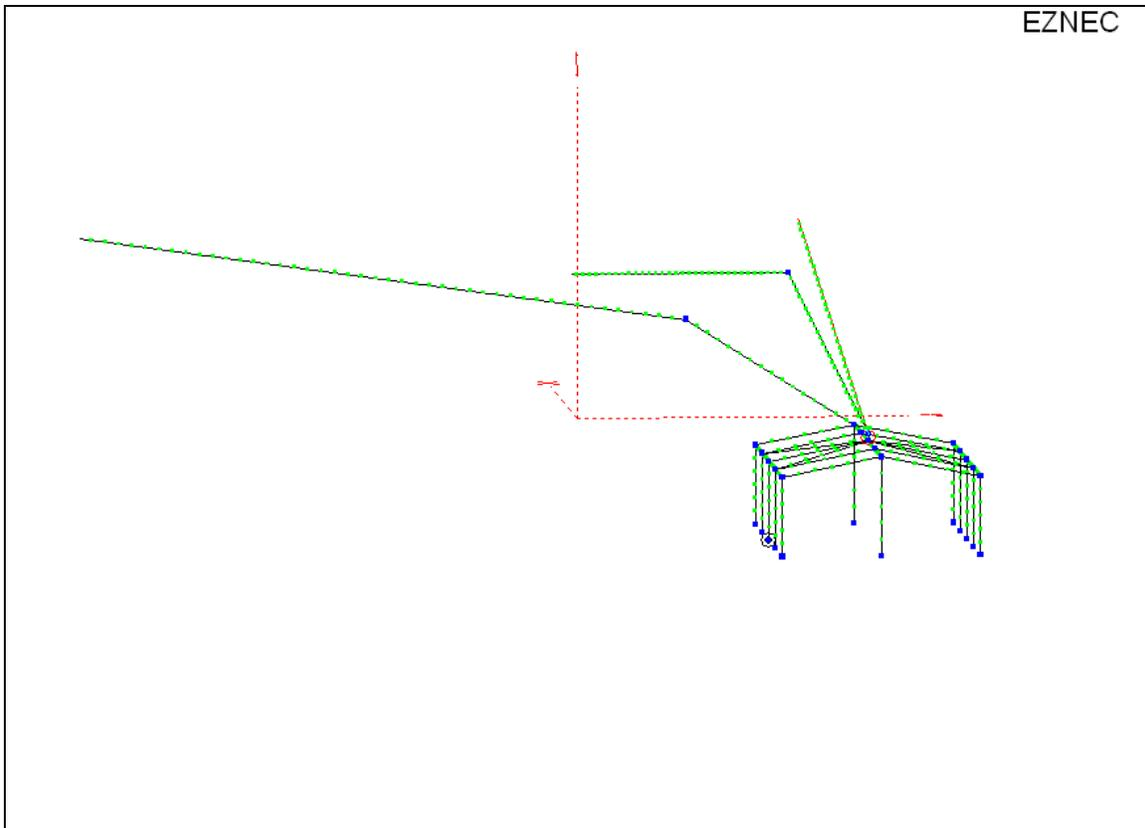
The graphic above shows the EZNEC definition I made for this antenna installation. As you can see, my barn is modeled as a wire frame with of the vertical lines, representing the sides of the barn, connected to ground.
