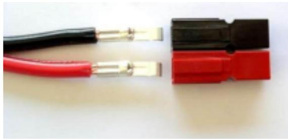
*Positioning contacts prior to insertion in contact bodies*
